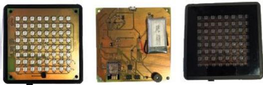
Fig. 1: (a) Frente PCB (b)Dorso PCB (c) Carcasa
