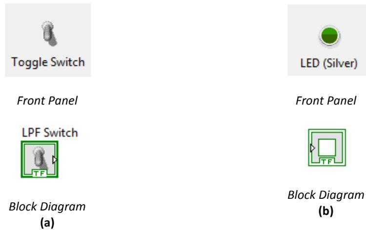
Fig. 35: Inserting the “Round LED” and “Vertical Toggle” Boolean Controls.
