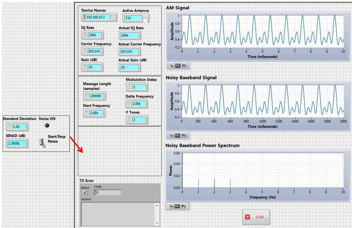
Fig. 127: Transmitter VI Template Front Panel
