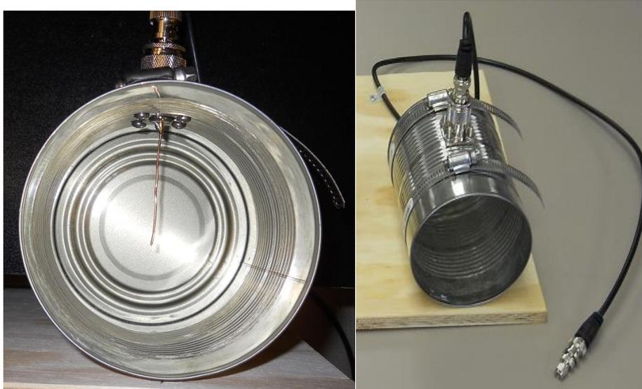
Fig. 225: Assembled Antenna
