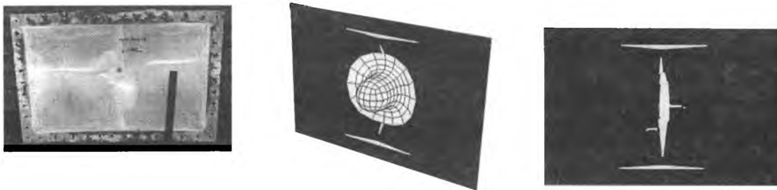
Figure 6. Comparison between numerical and predicted damage extension for bird impact at 147 m/s
