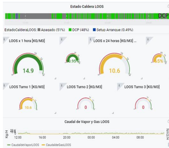
Fig.2. Dashboard that shows the status of a boiler from data gathered by the IIoT architecture. Source: Authors.
