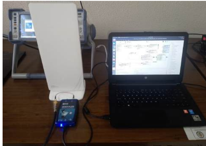
Fig. 1. One Seg receiver developed using software defined radio for ISDB-T One Seg, implemented in GNU Radio.
