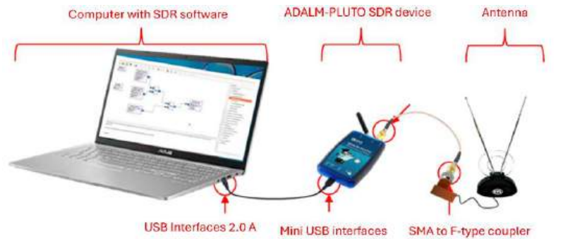
Fig. 1. illustrates the reception system used in this work, showing the signal path from the SDR to the MPEG-TS generation.
