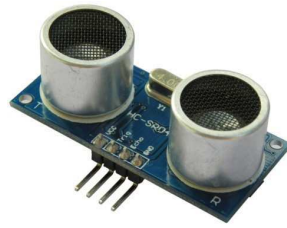
Fig. 1. Ultrasonic Ranging Module HC-SR04 [10]
